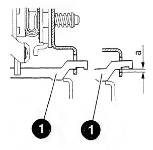
Adjusting control relay and starting-motor solenoid
